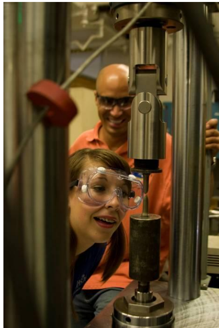
JASON Project student Argonaut Aubrey Gonzalez examines a metal rod being tested in a stress/ strain machine at NASA's Jet Propulsion Laboratory in Pasadena California as engineer Kobie Boykins looks on. © The JASON Project. All rights reserved.
